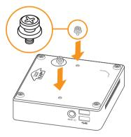
Align the D210 with the Mounting Plate so that indicator arrows on the plate and the decoder are pointed upward. Insert the heads of the extended screws on the D210 into the keyhole slots of the Mounting Plate and slide down to secure.
