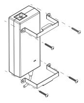
An optional VESA Mount Bracket Kit (910-0002-006) is available for applications where an encoder/decoder must be located on a VESA mount. The VESA Mount Bracket Kit (910-0002-006) includes a Wall Bracket that the can VESA Bracket can attach to.
