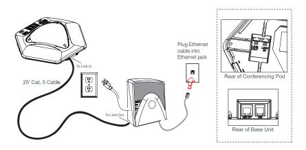
Warning: DO NOT plug a laptop or PC into the Link Out jack on the base unit or conferencing pod -- severe electrical damage can occur!
