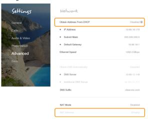
The COLLABORATE Live obtains its IP automatically by default from the DHCP server.
