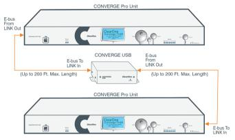
Note: Link Channel Selection is NOT required when the CONVERGE USB is used only as an E-bus extender with no USB Tx/Rx channels used.
