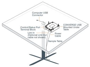
The CONVERGE USB Interface can also be placed near the CONVERGE Pro units or at any other location if care is taken to remain within the operational limits of the USB, power and E-bus cabling.
